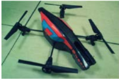
Figure 2. An AR.Drone quadcopter using outdoor hull.
